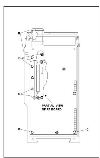
Figure 7 - RF Board Access
